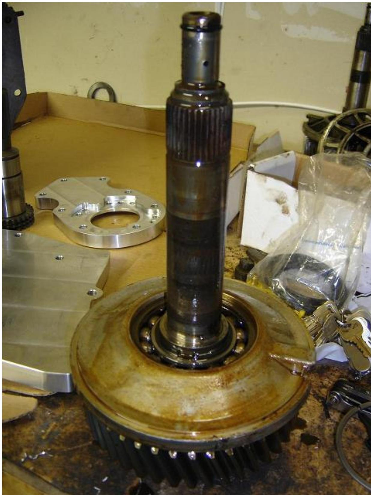
Remove the low range gear and intermediate shaft assembly by pulling it straight out of the range box, and place the assembly on the workbench.
