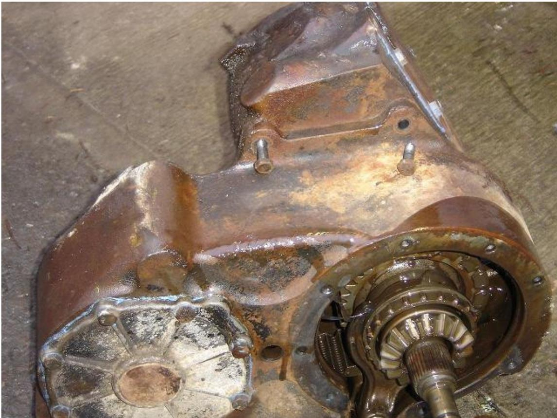
This may require a light tapping or wiggling on the chain case to break the gasket seal. Once you have the cases separated about 1" you will notice a rod hooked from the range box onto the rear shift rail. You will need to unhook this rod. Once you have, you can now lift the chain case up and away from the range box. This may require some wiggling to free.
