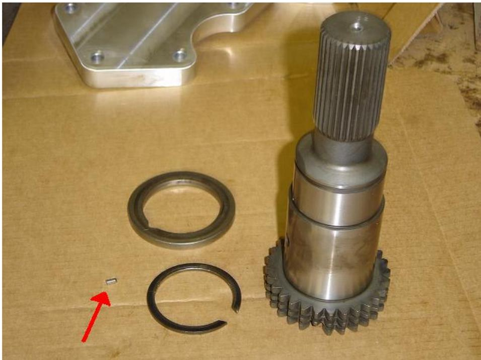
These are the parts you will need to keep for the re-installation of your low range gear and billet main shaft. Don't forget the locating pin!
