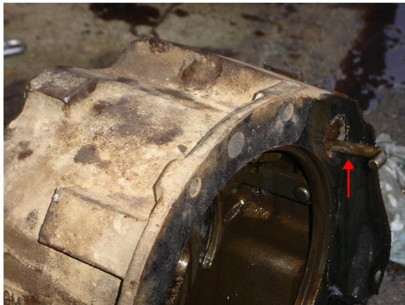
If you do not remove this, it could potentially fall into your range box and cause serious damage to your gears.
