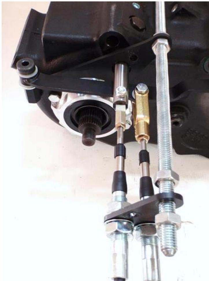
Use the 3/8"x1 1/4" cap screw, (3) 3/8" Nylon washers, and a 3/8" NC Stover nut to join the clevis yoke to the rocker arm.
