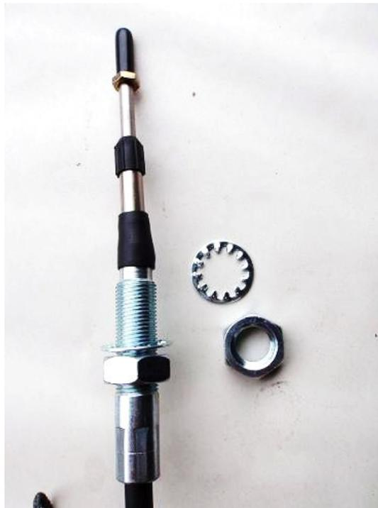
Now slide cable ends through bulkhead as shown. Reinstall locking ring and jam nut. Do not tighten down as these will have to be adjusted later.
