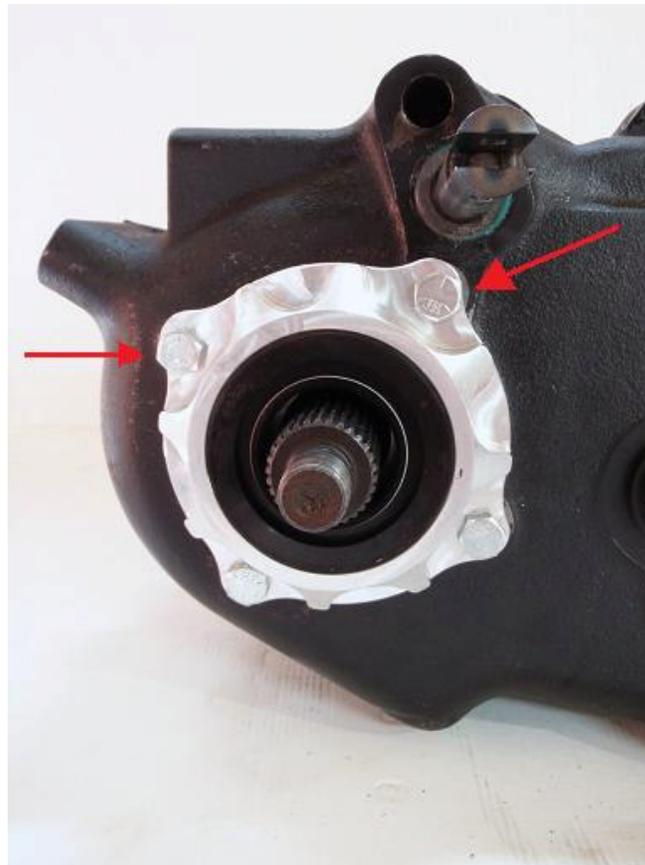
Position the Retainer mount over the NP205 Output as shown, and secure it in place with 3/8" x 1" NC Cap Screws.
