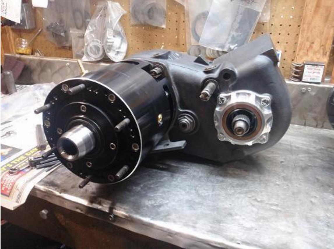
Important Note: Not all Transfer Cases use the same length Input Shaft, when test fitting the BlackBox to the Transfer Case make sure the BlackBox mates to the Transfer case with no gap. The most common problem people run into is the Input Shaft of their Transfer Case is too long and will bottom out against the rear Output Bearing before the BlackBox is fully seated. The most common gap to see is 3/4 of an inch.
