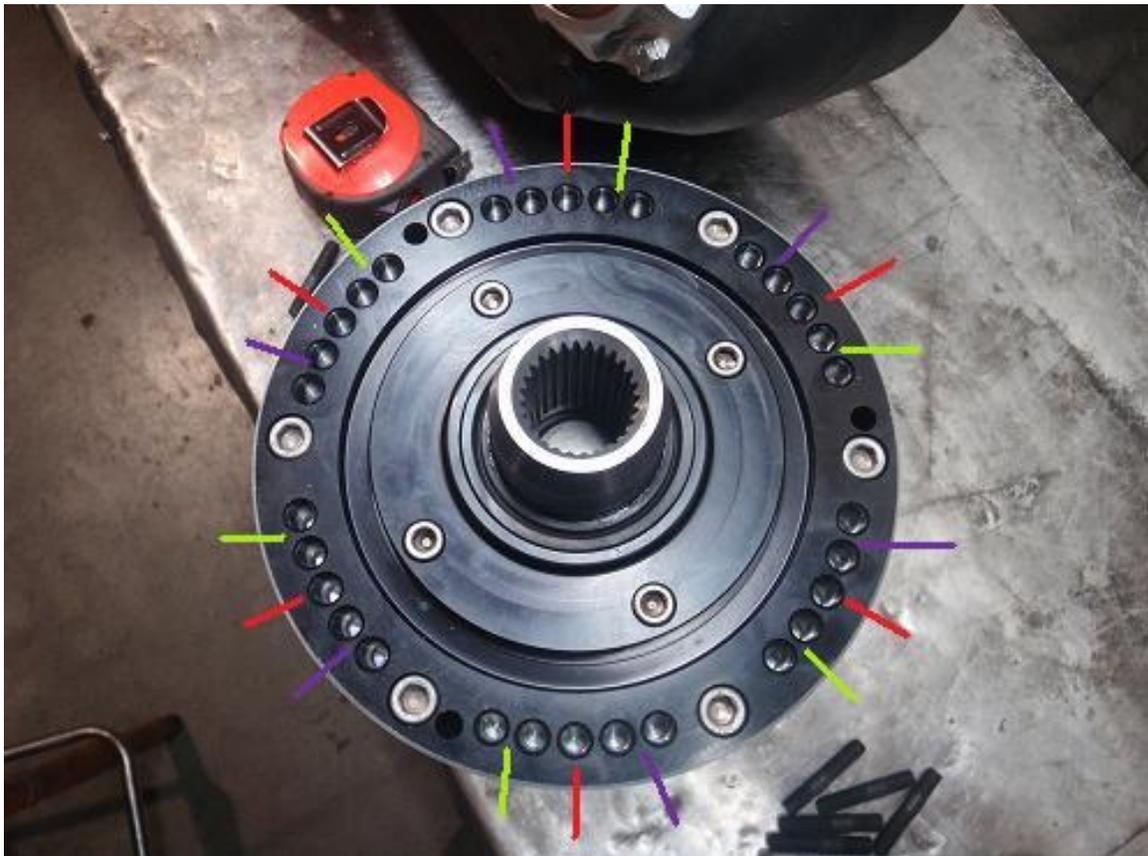
If you wish to clock your transfer case Clockwise (Viewing from the front) re-position the studs Counter Clockwise from the center position. (Purple Lines in Picture)
