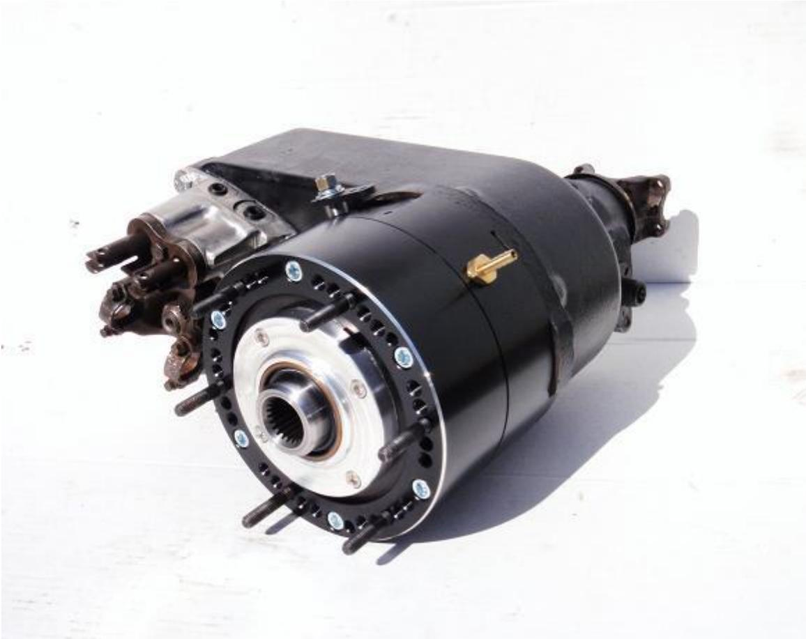
Thread the short coarse thread into the BlackBox-i by first locking two 3/8" NC nuts together on the stud, and turning the top nut with either a 9/16" wrench or socket.
